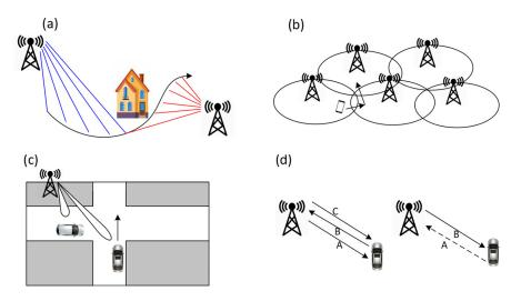
Figure 1. Application scenarios of mobility prediction in mobile networks: (a) positioning for millimeter wave beam sweeping; (b) small-cell hand over; (c) traffic management and self-driving cars; and (d) reductions of communication redundancy and overhead.
