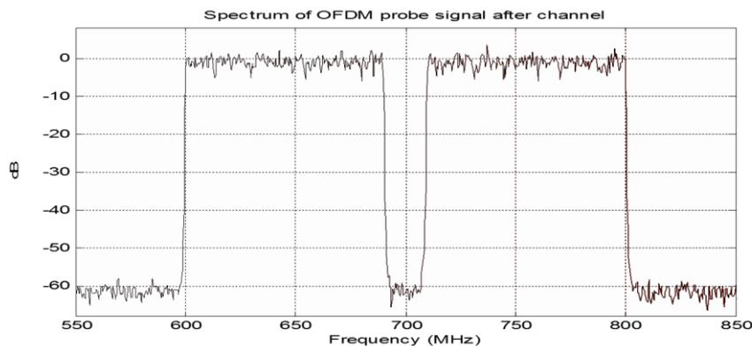
**Notch showing 10 MHz wide LTE Interference at -35 dBc**
